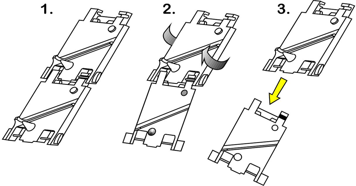
The following 3 sketches show how to assemble the 'track plate'.
