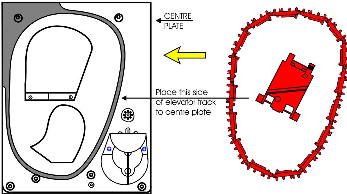
2. Once the 'track plate' is in position, turn the track through  $720^{\circ}$  to ensure it is seated in the guide path correctly.
