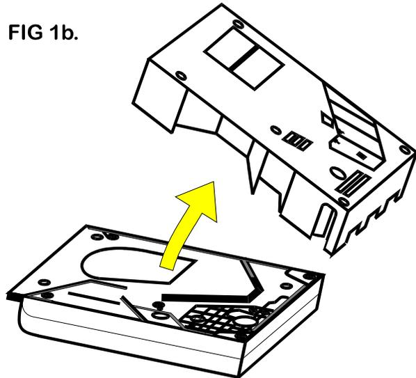
**ACCESS IS NOW AVAILABLE TO THE 'LOW LEVEL' SENSE PLATES, THE MAIN PCB, THE EXIT WINDOW, THE MOTOR TERMINALS & PART OF THE WIRING LOOM.**
